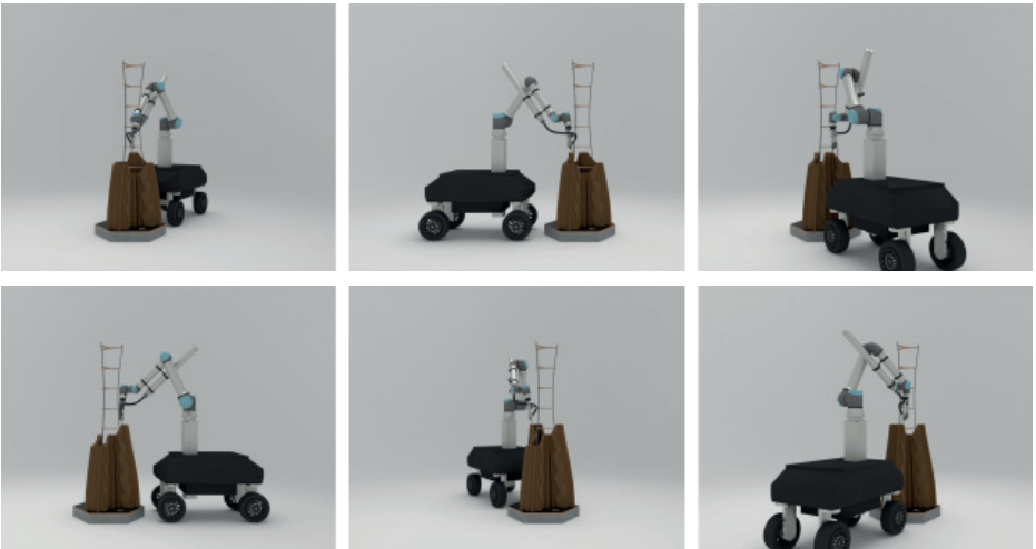
Figure 1: Succession of six mobile base locations for the manufacture of six respective segments around a reinforcement cage, followed by a cycle of filling the formwork with concrete after every three segments.
