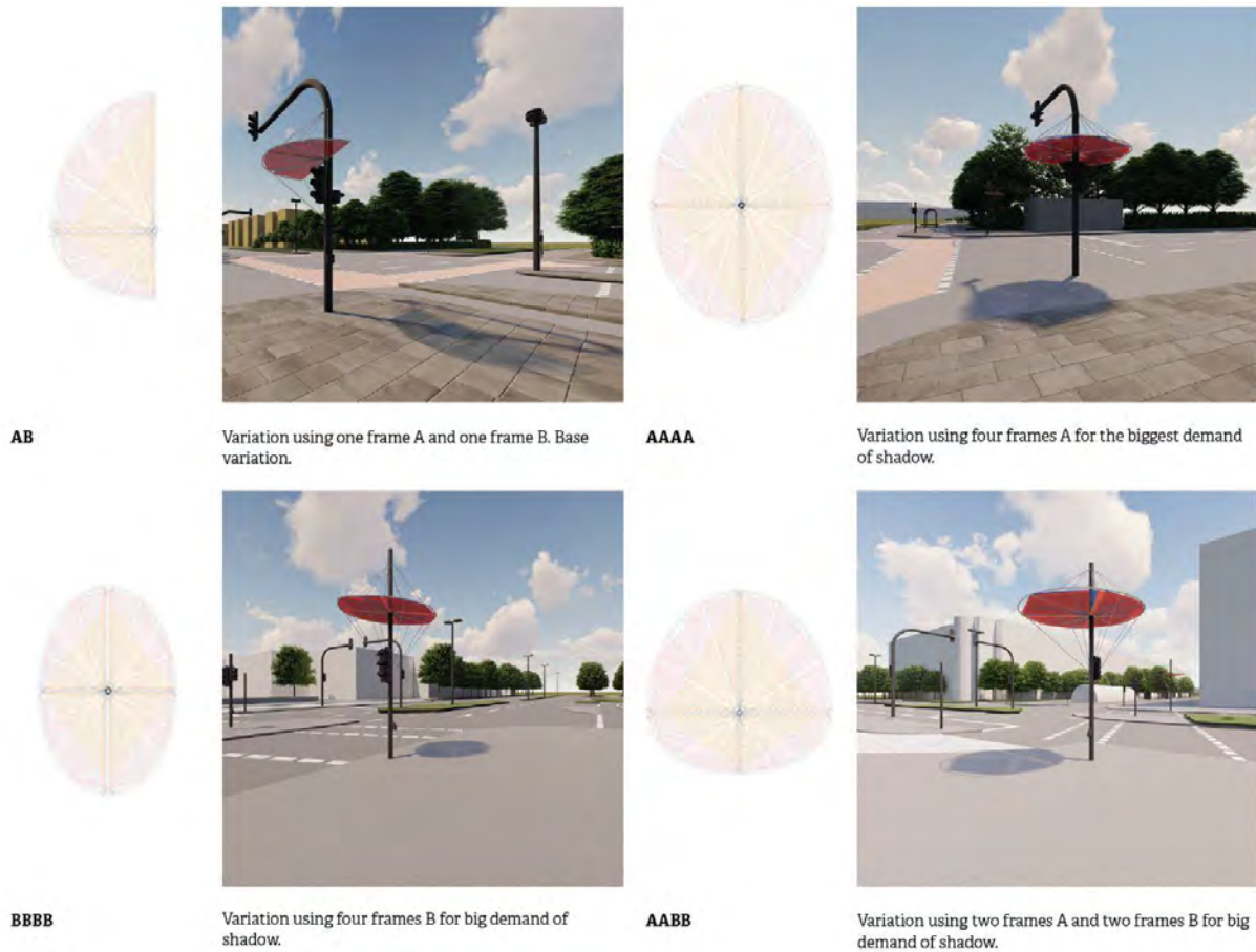
Figure 82 – Modular variations for two modular systems: a bigger (A) and a smaller (B) construction.
