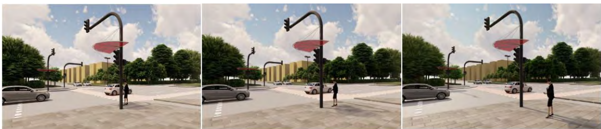
Figure 83 - Behavior simulation of moving shadow and temporal movement of the waiting area. From left to right: Position of shadow at 12:30 pm, 2:30 pm, and 4:30 pm.
