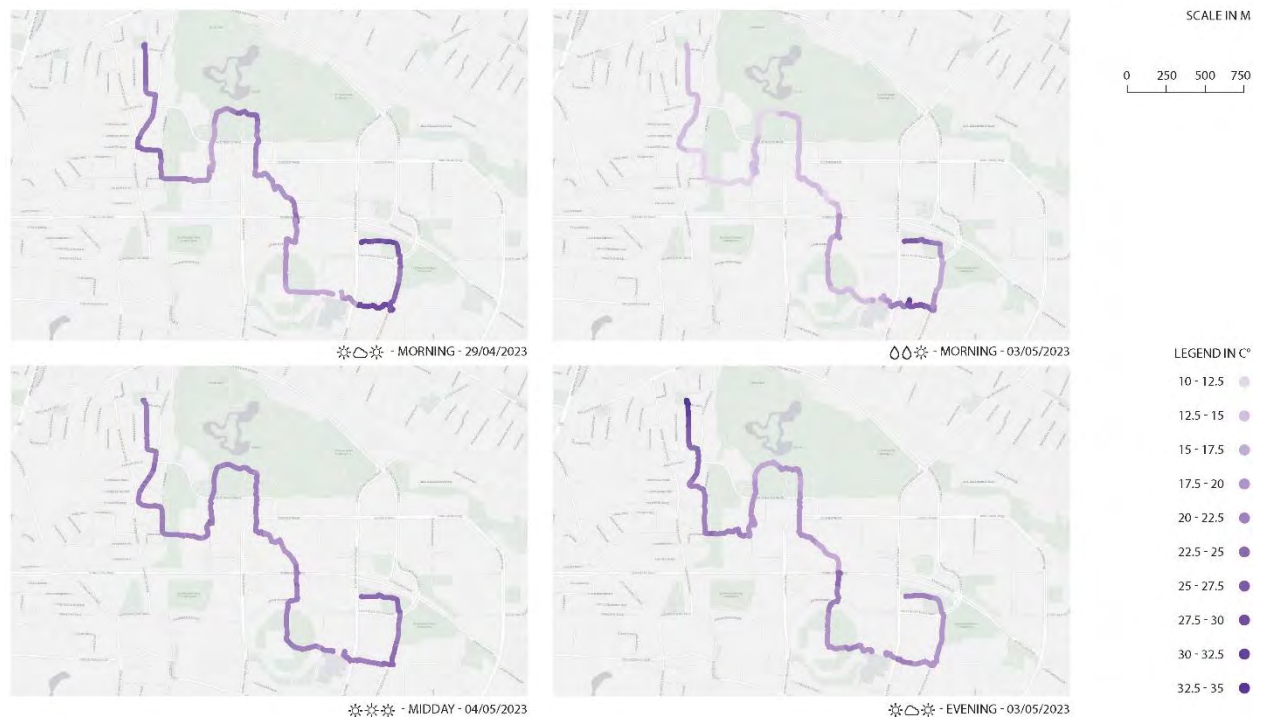
Figure 6 - Globe temperature (°C) A measure of temperature that considers radiant energy exchange. It is measured using a thermometer in a hollow, black, spherical globe.
