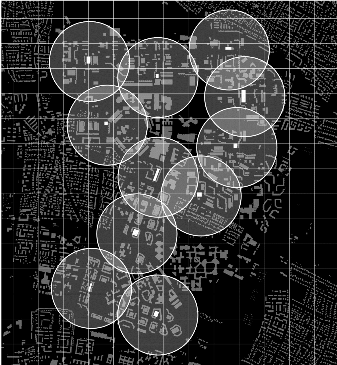
Figure 61 - Coverage with >10% of garages converted. With only 11 garages converted, almost every citizen of Neuperlach could be able to reach a converted underground space within only a few minutes of walking. (Radius = 400m).
