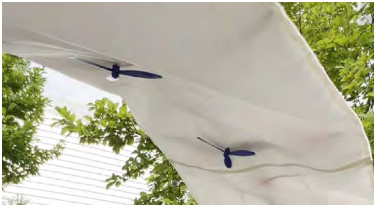
Figure 65 - Integrated and solar powered fans.
