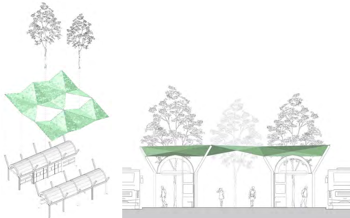
Figure 40 – Axonometry (left) and Section (right). Overarching roof structure made of braided panels over the existing shelter structure.
