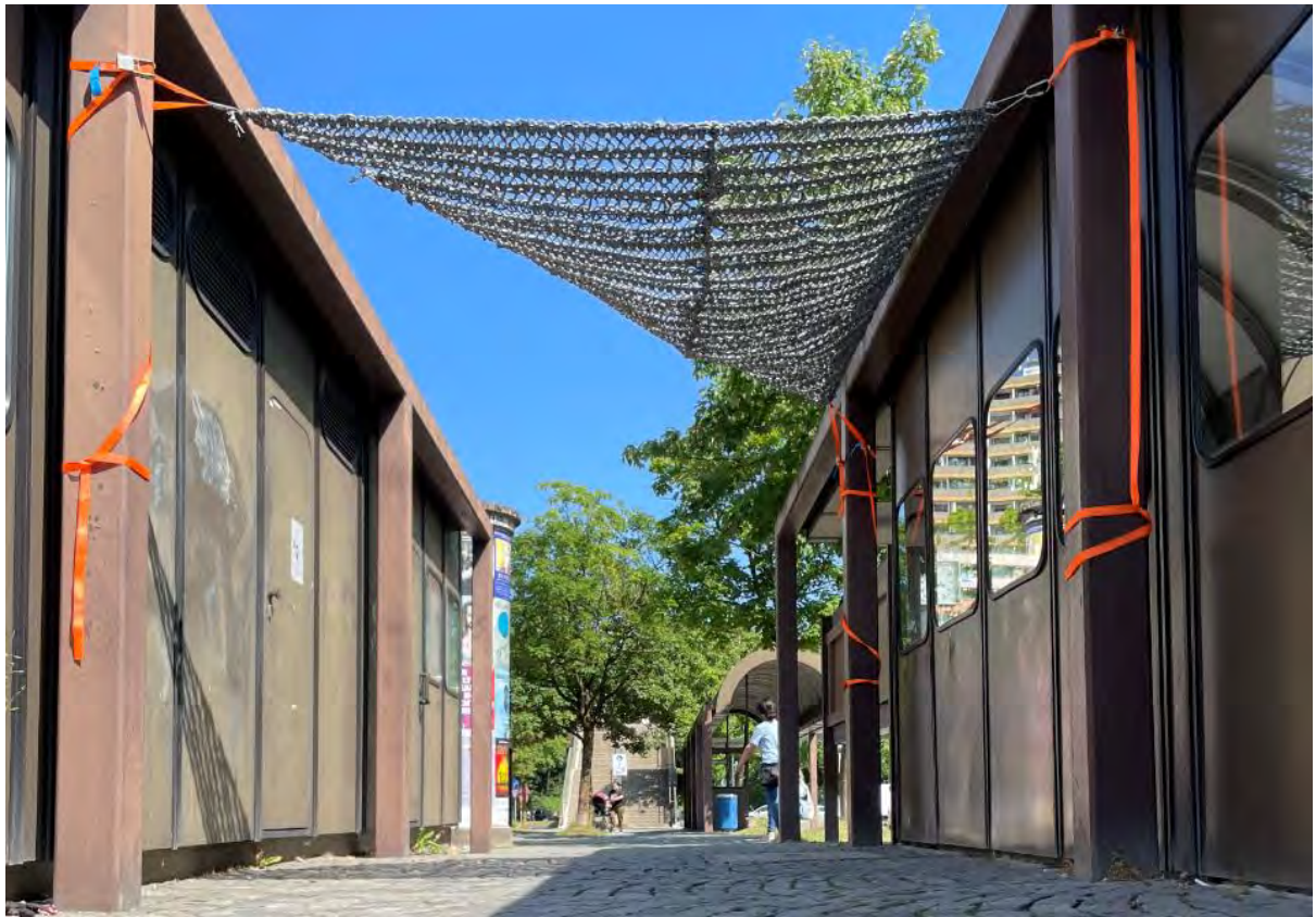
Figure 44 - Demonstrator testing set up. Mounting with carabiners and ratchet straps.
