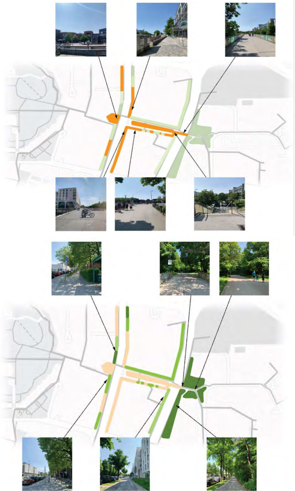
Figure 24 – Conceptual shading map identifying areas of shade through vegetation (green) and built surroundings (orange). The darker the green color coding the denser the shade.
