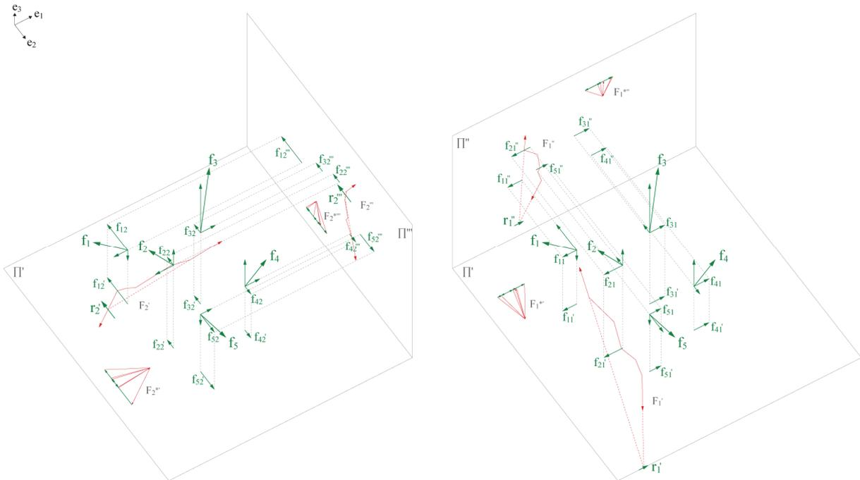
Figure 6: Determination of  $\mathbf{r}_2'''$  on  $\Pi'''$  and  $\mathbf{r}_2'$  on  $\Pi'$  (left); determination of  $\mathbf{r}_1'''$  on  $\Pi'''$  and  $\mathbf{r}_1'$  on  $\Pi'$  (right)
