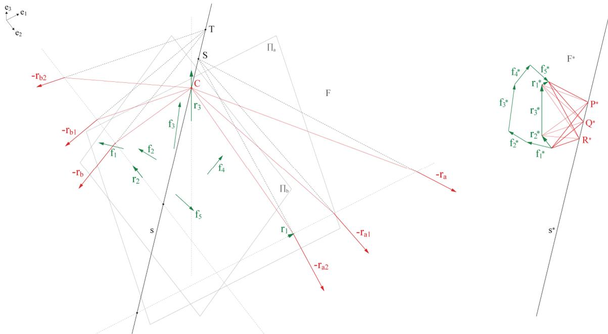
Figure 9: Construction of pairs of conjugate forces belonging to the planes  $\Pi_a$  and  $\Pi_b$
