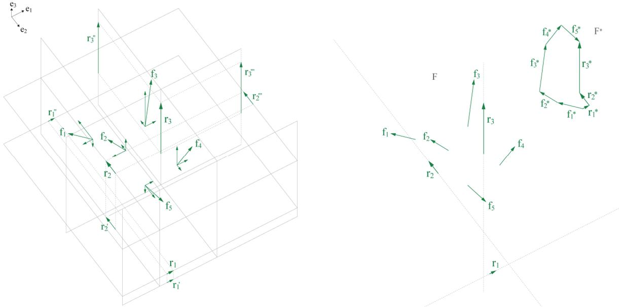
Figure 7: Determination of  $\mathbf{r}_1, \mathbf{r}_2$  and  $\mathbf{r}_3$  (left); the given system of forces  $\Sigma$  with the resultants  $\{\mathbf{r}_1, \mathbf{r}_2, \mathbf{r}_3\}$  (right)
