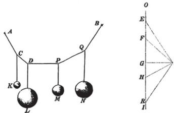
Figure 1: Funicular structure and force polygons by Varignon [13]
