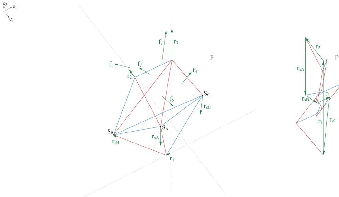
Figure 11: Evaluation of the reactions  $\mathbf{r}_{sA}, \mathbf{r}_{sB}$  and  $\mathbf{r}_{sC}$  at the supports (red-tension, blue-compression)
