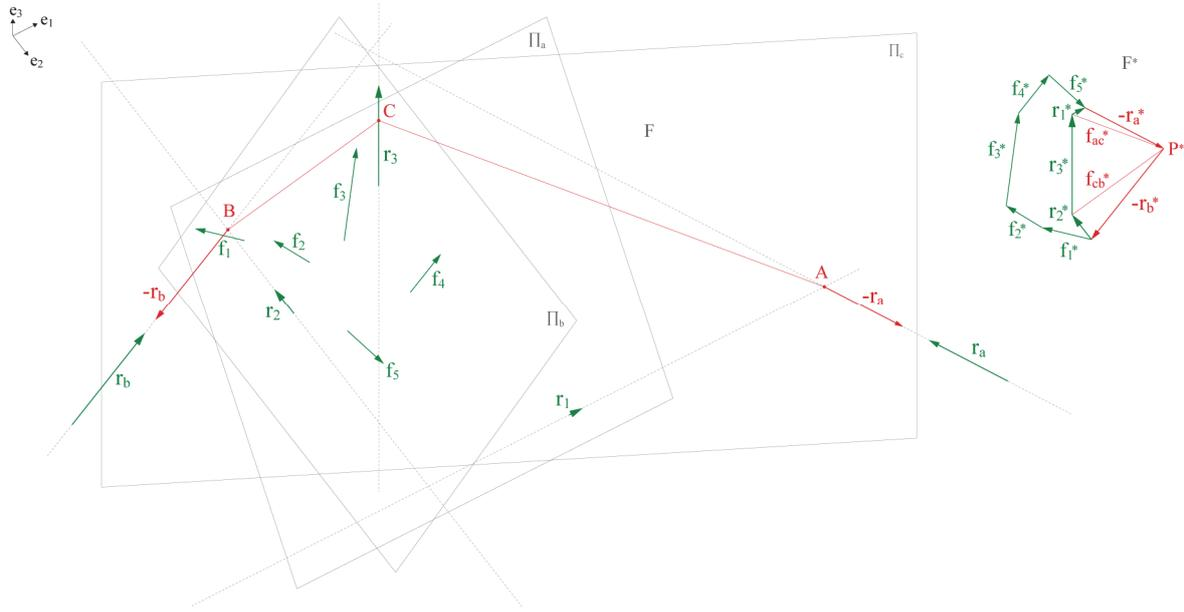
Figure 8: Composition of three skew resultants  $\{\mathbf{r}_1, \mathbf{r}_2, \mathbf{r}_3\}$  into two resultants  $\{\mathbf{r}_a, \mathbf{r}_b\}$
