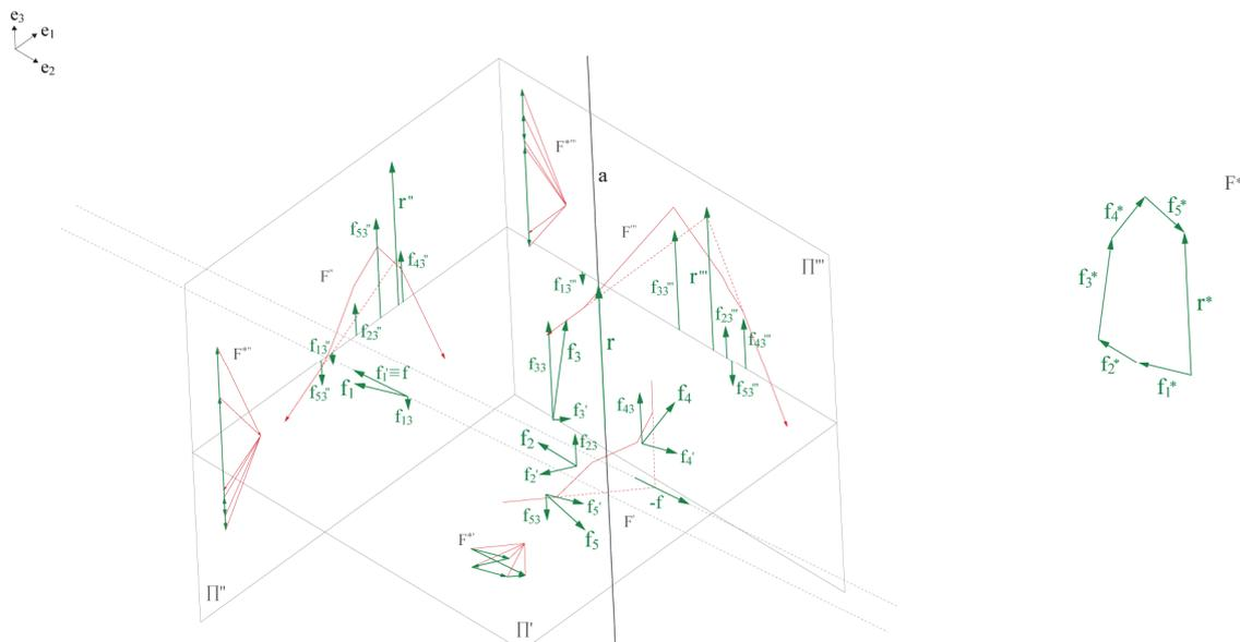
Figure 10: Determination of one resultant and one couple of  $\Sigma$
